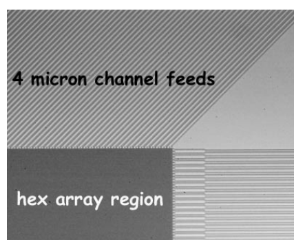
Figure 5. A corner of an N -port array showing the array of channels feeding into an open area consisting of a hexagonal array of 2\ \mu\text{m} posts. The width of the narrow channels feeding fluid into the array is 4\ \mu\text{m} .
