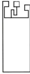
Figure 3. A three-port injector. The centre channel has a width of 10\ \mu\text{m} and the two wide side channels have widths of 100\ \mu\text{m} . The entire device is 7\ \mu\text{m} deep
